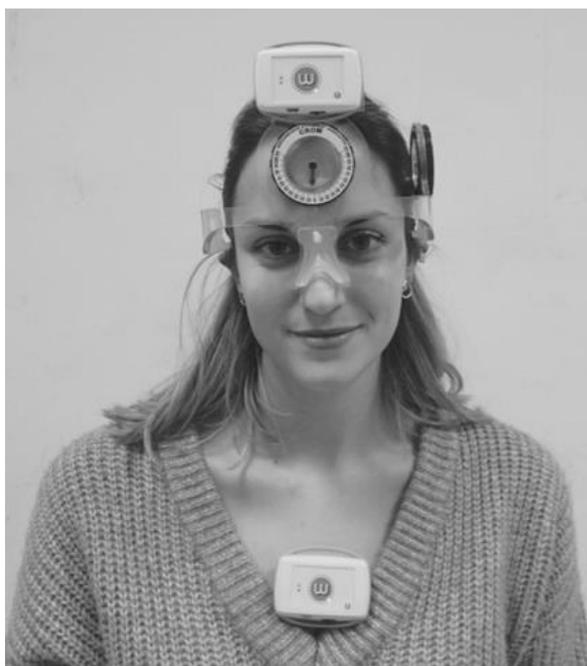
**Figure 1:** Simultaneous localization of the inertial sensors and the CROM instrument
